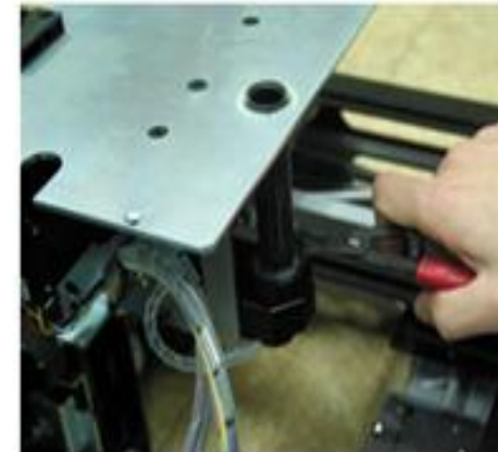
[Replacing consumable part (Rubber tee) image]
